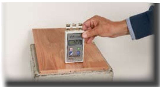
Scanning Depth 10 mm - Measures only the Wooden Floor
